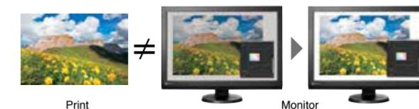
Adjust the **2 White Point**. Move the pointer to the left or right until it approximates the appearance of the print. If the screen output seems blue, move the pointer away from the blue spectrum and toward the red end of the spectrum to remove excess blue.
